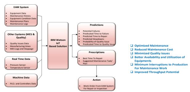
(OEE). The overall equipment effectiveness is impacted by availability loss due to downtime, performance loss due to equipment condition, quality loss due to defective part production. The improvement in these areas can improve the OEE and hence the production rate.
